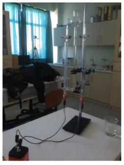
Figure 1: The Electrolysis Apparatus
