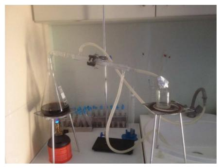
Figure 4: Distillation of Contaminated Water
